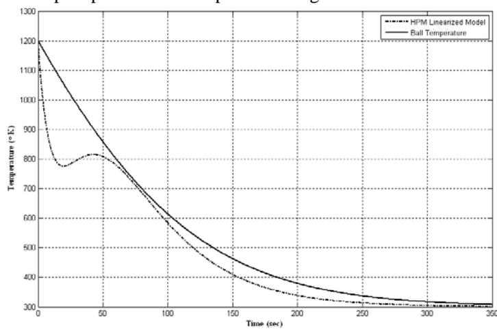
Figure 7: The ball and the HPM linearized model temperature, considering a 3<sup>rd</sup> order approximation of  $\nu$
