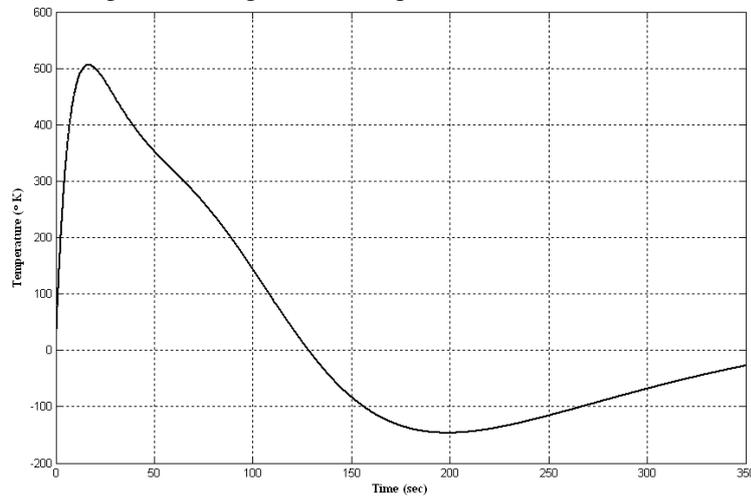
Figure 9: The temperature error between the linearized model by homotopy perturbation method and the nonlinear model in a closed loop PI controlled (a 3<sup>rd</sup> order approximation of  $V$  is considered).
