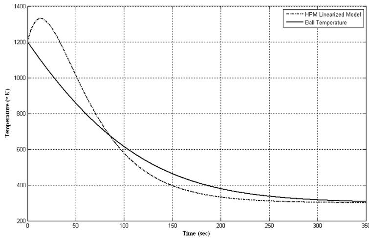
Figure 3: The ball temperature and the estimated behavior according to HPM, considering a 2<sup>nd</sup> order approximation of  $\nu$
